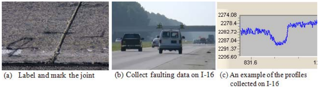
8 9 Figure 7 Field test conducted on I-16.
