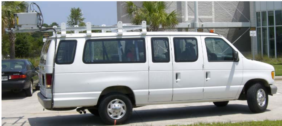
Figure 2 The sensing van for collecting faulting data.
